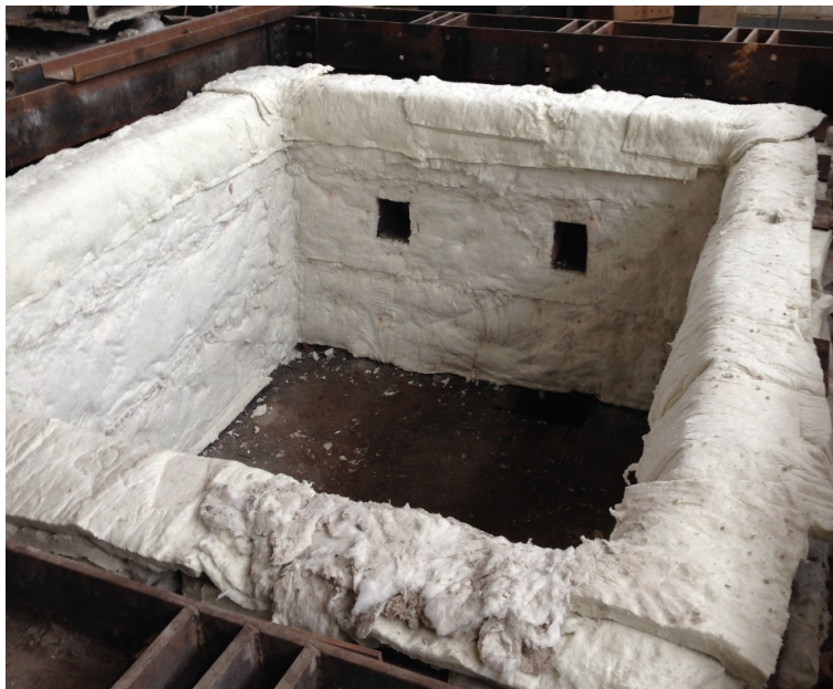
(b) External view of the self-designed furnace
