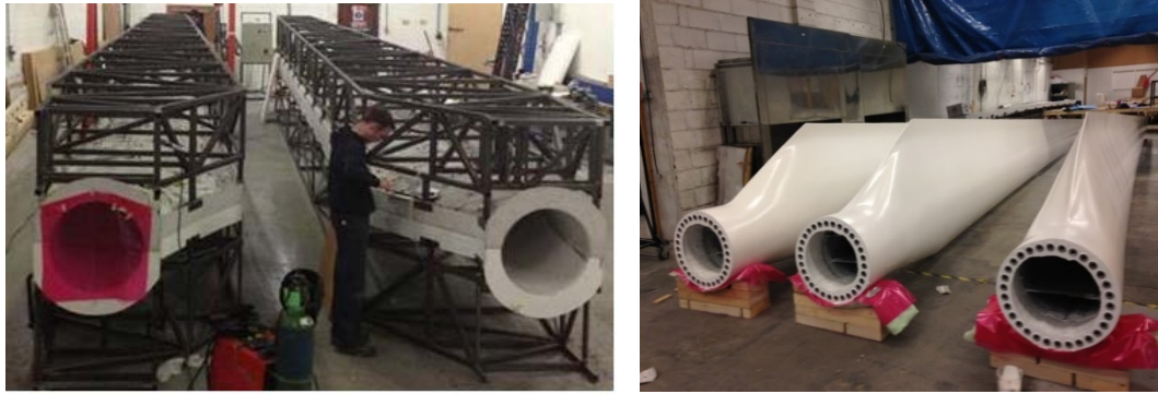
Fig. 2. Ceramic heated tools (left); and 12.6 m blades made from epoxy powder based VBO prepreg (right).
