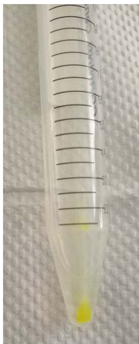
Figure S14. The demonstration of successful conjugation of PEG to ZIF-8 nanocomposite. (In order to demonstrate successful conjugation of PEG to ZIF nanocomposites, we labelled PEG with FITC to track PEG molecules after reaction. In the experiment, FITC labelled PEG molecules were mixed with ZIF-8 nanocomposites; after reaction, the nanocomposites were centrifuged. If PEG was not successfully conjugated to the nanocomposites, the fluorescent PEG molecules would be remained in the solvent. It was found that almost all fluorescence signal was from the precipitated ZIF-8 NMOFs nanocomposites, indicating the successful conjugation of PEG to ZIF-8 nanocomposites.)
