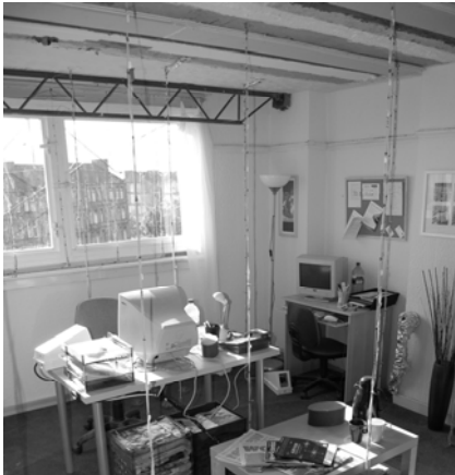
(a) Fire compartment, with FRP at top
