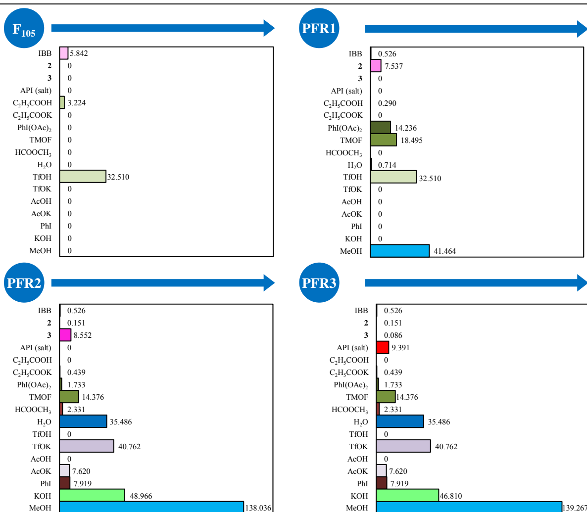
Figure 4. Continuous ibuprofen synthesis mass balance at key flowsheet points [25].
