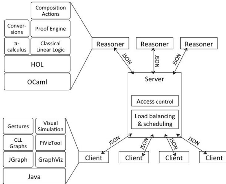
Fig. 4: The 3-tiered server-client architecture of WorkflowFM.
