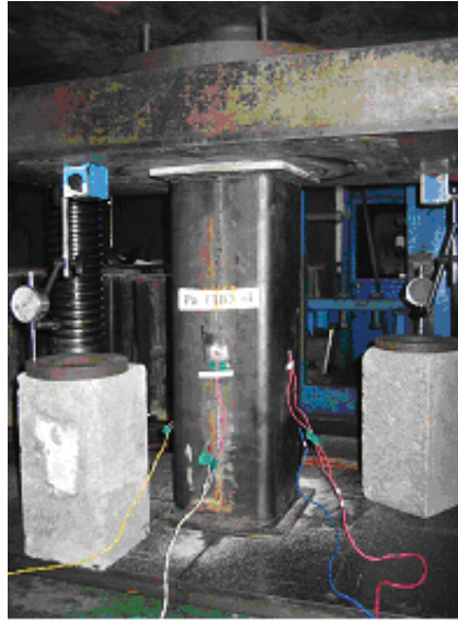
Fig. 4. Test setup of CFST-composite column specimen
