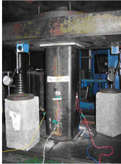
Fig. 4. Test setup of CFST-composite column specimen
