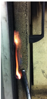
Fig 9. Testing leaked gases
