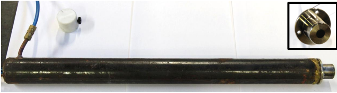
Figure 10 – Schmidt-Boelter heat flux gauge mounted on a self-cooling probe system designed to minimise the influence of convective flows near the gauge.
