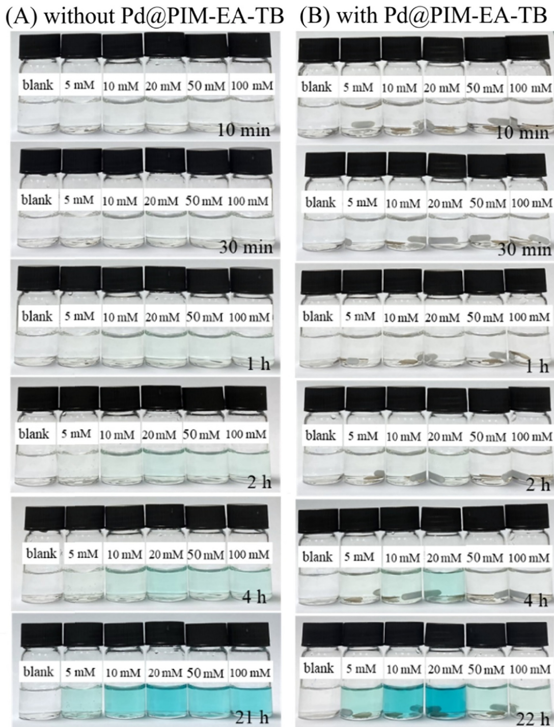
Fig. 11. (A) Effect of HCOOH/HCOONa concentration at pH 3.75 on TMB reactivity. Photographs of 580 \mu\text{M} TMB the absence of Pd@PIM-EA-TB (stirred in the dark, 33 % DMSO) as a function of reaction time. \text{H}_2\text{O}_2 was added to reflect reactivity as in data presented in Fig. 7C: blank: no \text{H}_2\text{O}_2 , 5 mM: 33 \mu\text{M} , 10 mM: 41 \mu\text{M} , 20 mM: 59 \mu\text{M} , 50 mM: 111 \mu\text{M} , 100 mM: 198 \mu\text{M} \text{H}_2\text{O}_2 . (B) Photographs of 580 \mu\text{M} TMB the presence of Pd@PIM-EA-TB (stirred in the dark, 33 % DMSO) as a function of reaction time. \text{H}_2\text{O}_2 was generated in situ .
