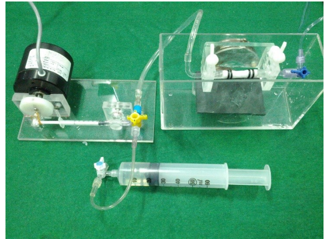
Fig. 6. The fully assembled phantom system with drive motor and water tank.
