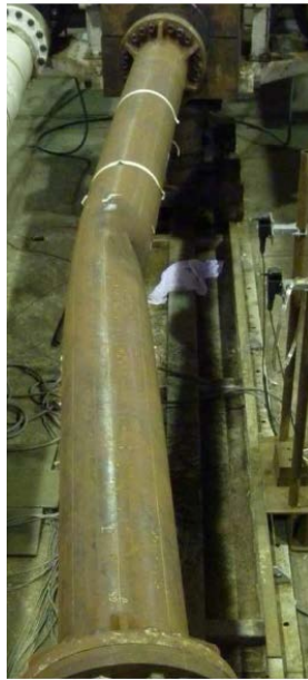
Figure 10. Beam-column BL-50 after testing
