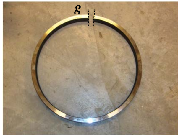
Figure 2. (a) Device for measuring initial wrinkling of tube wall; (b) Ring specimen extracted from \varnothing 355.6/12 tube after splitting.
