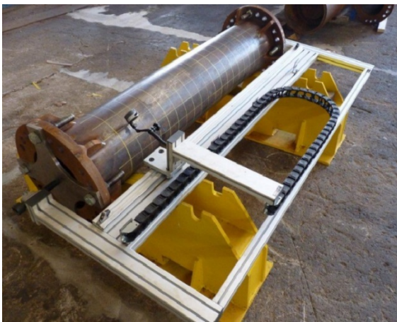
Figure 2. (a) Device for measuring initial wrinkling of tube wall; (b) Ring specimen extracted from \varnothing 355.6/12 tube after splitting.
