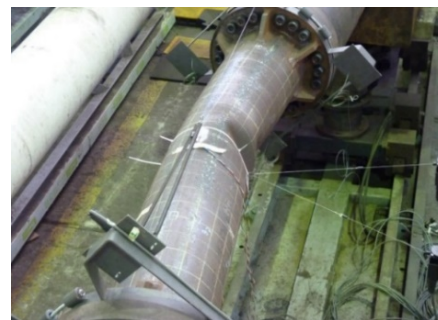
Figure 7. Buckled specimens under combined loading tests; specimen (a) BS-13 and (b) BS-75.
