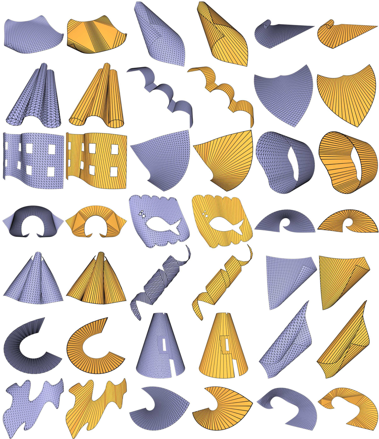
Fig. 24. Various remeshing results obtained with our method. Note that our method can handle a wide variety of developable geometry and topology, including cylindrical topology, multiple holes, and sophisticated boundary shapes.
