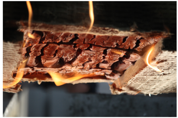
Fig. 13. Close-up of the heated zone of a beam during the test.
