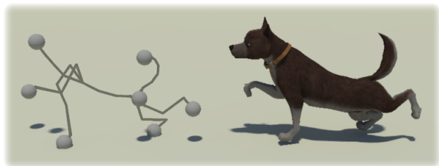
Fig. 5. Result of Rig-space Full Body IK. From seven end effectors placed at four feet, head, hip, and tail, the optimal rig attributes are approximated by GPR and the solution is further refined by gradient descent. The animators can interactively pose the character using seven end effectors while the rig attributes are updated in real time.
