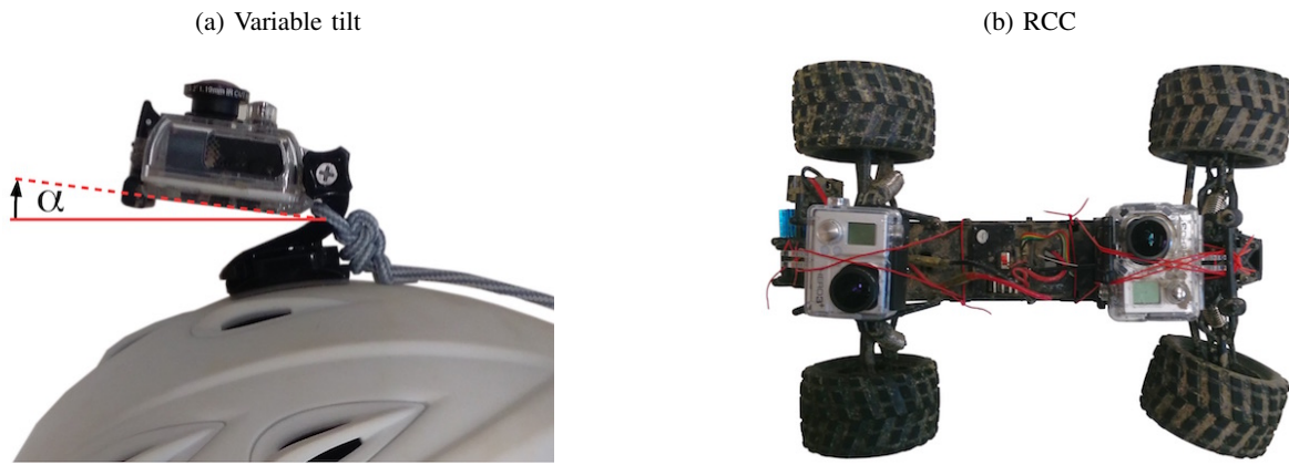
Fig. 2: (a) Side-view of the bicycle helmet setup with a single camera mounted at each run. The additional tilting is denoted by the angle \alpha , where \alpha = 0 with the camera approximately level. (b) Top-view of the RCC platform mounted with the RGB and UV cameras simultaneously, both pointing upwards.
