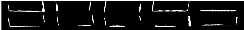
Figure 10: This is an example of the obtained dataset for the images shown in Fig. 5. Each of the previous insert gray-scale images with masked background follow a preprocessing step that yields four new images, one for each cutting edge in horizontal position.
