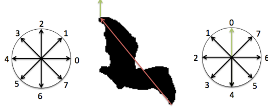
Figure 4: Example of the Boundary Orientations Chain (BOC) rotation invariance. The red arrow represents the maximal distance between points in the contour of the image. The green arrow is the orientation of the first point of the chain. The values assigned to each orientation are shifted locating the green arrow in the top of the diagram (value 0).
