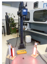
Figure 7: Image capture prototype. The support in which the camera is placed and the LEDs bars employed are shown.
