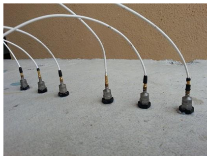
Figure 2. Photograph of accelerometer sensors arranged on the upper side of concrete specimen.
