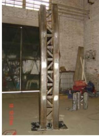
**Fig.18 LCFST column connected by lacing bars**
