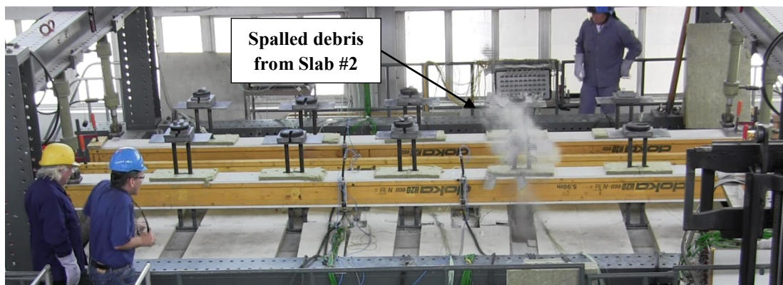
Figure 19 – Explosive spalling and immediate collapse of Slab #2 at 12' 37".
