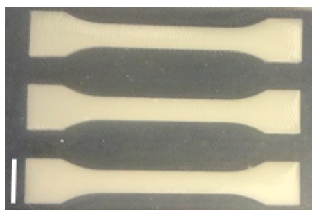
Fig. 6. To prepare hydrogel samples for tensile testing, PDMS ‘dog-bone’ moulds (890 \mu L volume) were used (scale bar 10 mm). The moulds were filled with the first network components, photo-polymerised, and then submersed in a solution containing the second network components and photo-polymerised again to create the double-network hydrogels.
