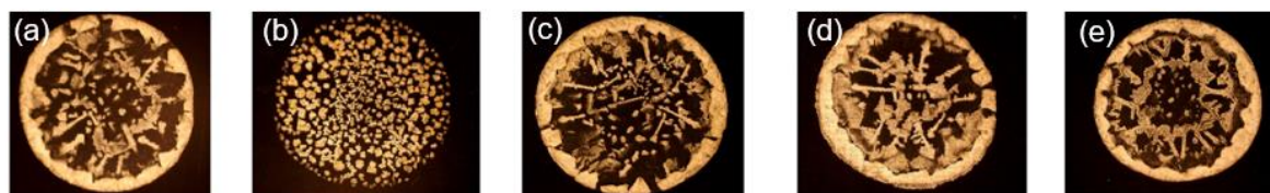
Fig. 19. Dried drop patterns from tequila adulterated with four different substances: (a) a control, (b) MEG (5 %v/v), (c) EtOH (10 %v/v), (d) Water (10 %v/v) and (e) MeOH (40 %v/v). From (87).
