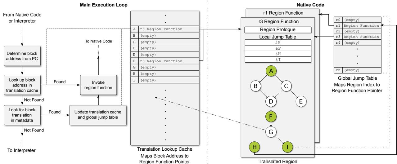
**Figure 5.** Interaction between regions via the *global jump table* and the internal interactions between basic blocks, either directly or via the *local jump table*. The control flow graph represents the region in the shaded area in Figure 4(B).
