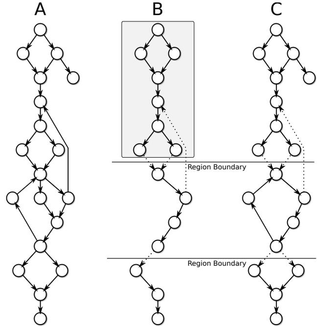
**Figure 4.** (A) Example of a whole-program control flow graph. (B) Parts of the control flow graph from (A) dynamically discovered after some time of execution, including forced region limits at page boundaries. (C) Additional control flow has been dynamically discovered after some more time executing the program.
