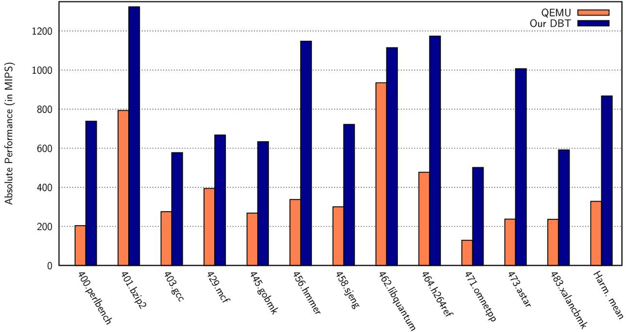
**Figure 7.** Absolute performance figures (in MIPS) for the *long-running* SPEC CPU2006 integer benchmarks for both QEMU-ARM and our DBT, indicating that the quality of the generated code by our system is superior to the code generated by QEMU-ARM.
