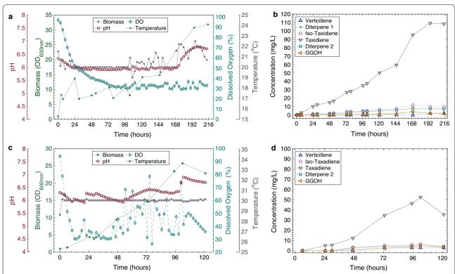
**Fig. 7** Bioreactor studies results and respective taxane concentration kinetics at 20 °C (**a, b**) and at 30 °C (**c, d**). LRS5 was cultivated in an Applikon MiniBio 500 bioreactor in yeast extract (1%), peptone (2%), galactose (2%). The pH and dissolved oxygen were monitored online and controlled to set points of 6 and 30%, respectively online
