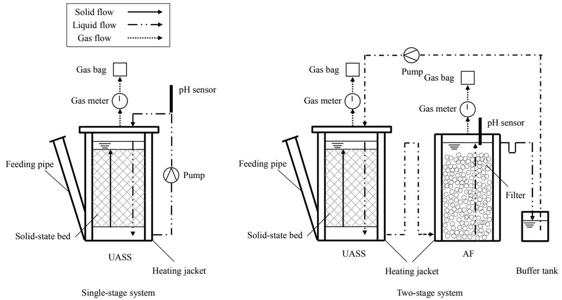
Fig. 1 - Schematic of the single-stage system and two-stage system. (UASS: upflow anaerobic solid-state reactor; AF: anaerobic filter).
