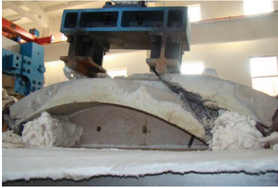
(c) HFRC2 ( P_v/R_H=1.2 , under fire )
