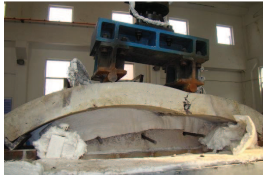
(a2) HFRC1, Under fire, free slide ( R_H=0 )
