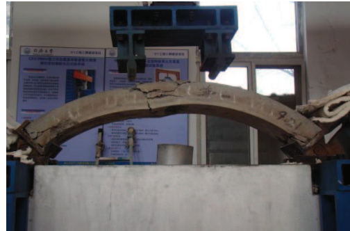
(b) RC4, Post fire, fixed pin ( d_H=0 )
