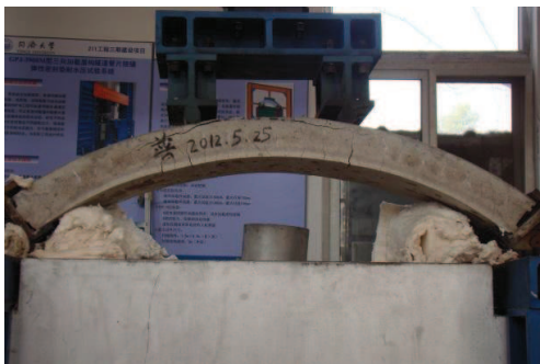
(a3) RC5, Post fire, free slide ( R_H=0 )
