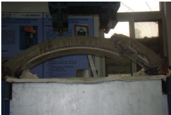
(a) RC2 ( P_v/R_H=1.2 , under fire)
