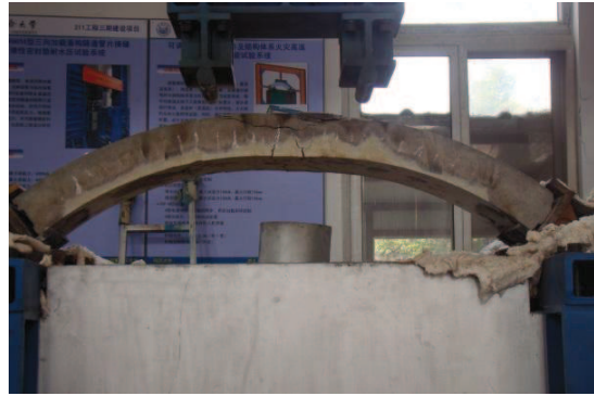
(a2) RC1, Under fire, free slide ( R_H=0 )
