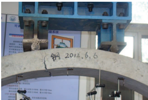
(a1) HFRC0, Ambient, free slide ( R_H=0 )
