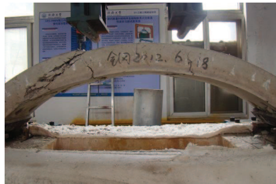
(b) HFRC4, Post fire, fixed pin ( d_H=0 )
