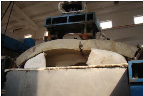
(a3) HFRC5, Post fire, free slide ( R_H=0 )
