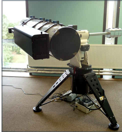
Figure 2: The laser system mounted on the telescope. A diagram of the system is shown in Figure 1.
