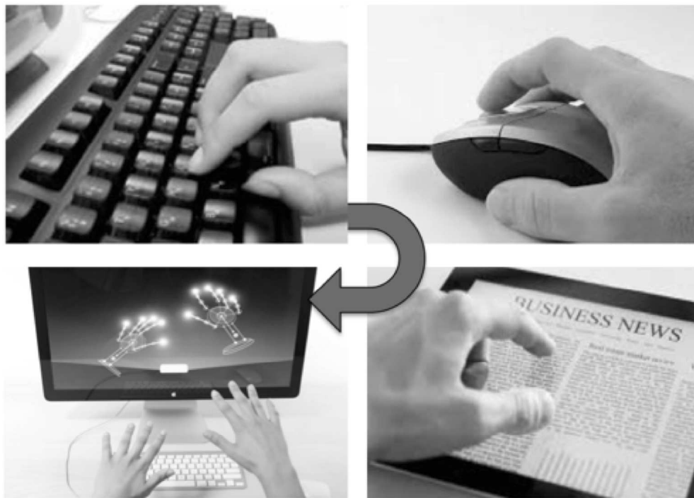
Figure 1. The spectrum of computer-user interfaces from keyboard to gesture interface, via mouse and touch screen. LEAP (bottom left) is a commercially available gesture interface device. 176x127mm (300 x 300 DPI)
