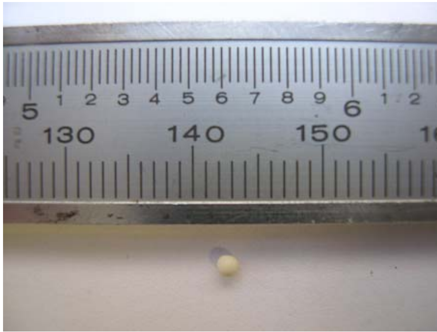
Figure 2: Particle size of 13X bead used in the ZLC experiments ( R = 0.8 mm)
