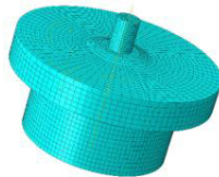
Fig. 1: FE model of the UCD.
