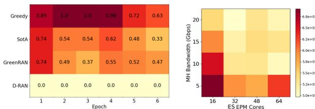
Fig. 6. Left: Heatmap showing fraction of vRAN functions processed at CS at 6 different adaptive intervals on 32 core EPMs and 15 Gbps MH bandwidth. Right: Heatmap showing total energy consumption ( $E_{\text{tot}}(t)$ , in  $KJoules$ ) for different combinations of ES configurations and MH bandwidths.
