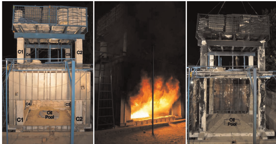
Fig. 6. (a) Simulated earthquake loading, (b) fire test and (c) residual capacity test on fire damaged RC frame.
