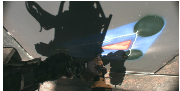
Figure 16: Top left: head camera view of poker used to press drill's power button. Top right: visualization of the nominal plan to reach all drill target points in the triangle. Bottom right: head camera view provides situational awareness to operator as robot executes drilling plan. Bottom left: Robot avatar and RGB point cloud visualization with affordance models of the drill and triangle target.
