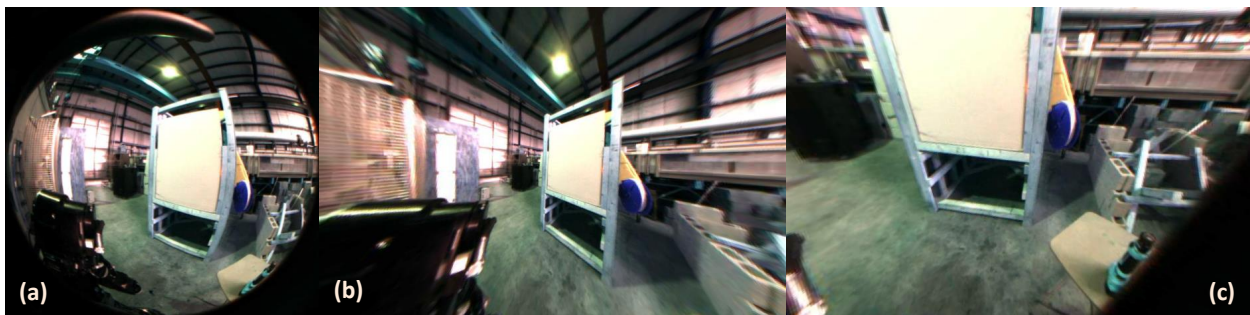
Figure 4: Fisheye lens rectification. (a) Raw image from left chest camera exhibits severe fish-eye distortion and is difficult to interpret at the periphery. (b,c) After lens calibration, images can be rectified to produce arbitrary virtual viewpoints with minimal distortion.
