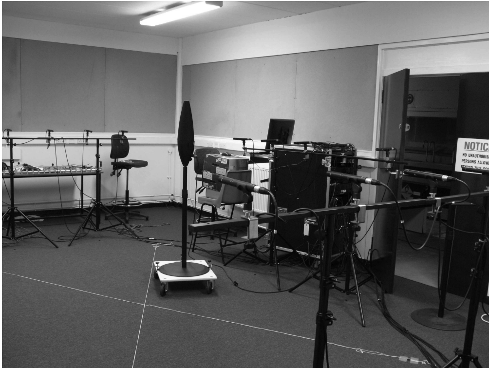
Figure 7: Real audio room environment for performance evaluation. The laboratory is located at the University of Edinburgh, Scotland. The room has carpet floor, concrete block walls and ceiling, and glass windows covered by hard cardboard with a thickness \approx 0.4\text{cm} . The measured reverberation time is 0.836\text{s} and the ambient noise level is -40\text{dB} [42].
