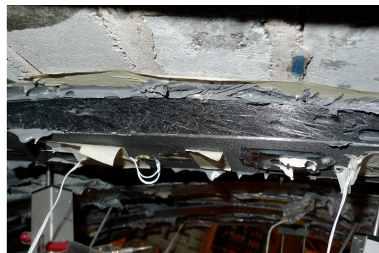
(a) Shear crack and debonding at Plate P_{N1} (b) Flexural crack and debonding at Plate P_{S4}
