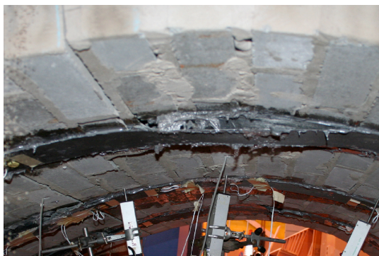
(a) Shear crack and debonding at Plate P_{N1} (b) Flexural crack and debonding at Plate P_{S4}
