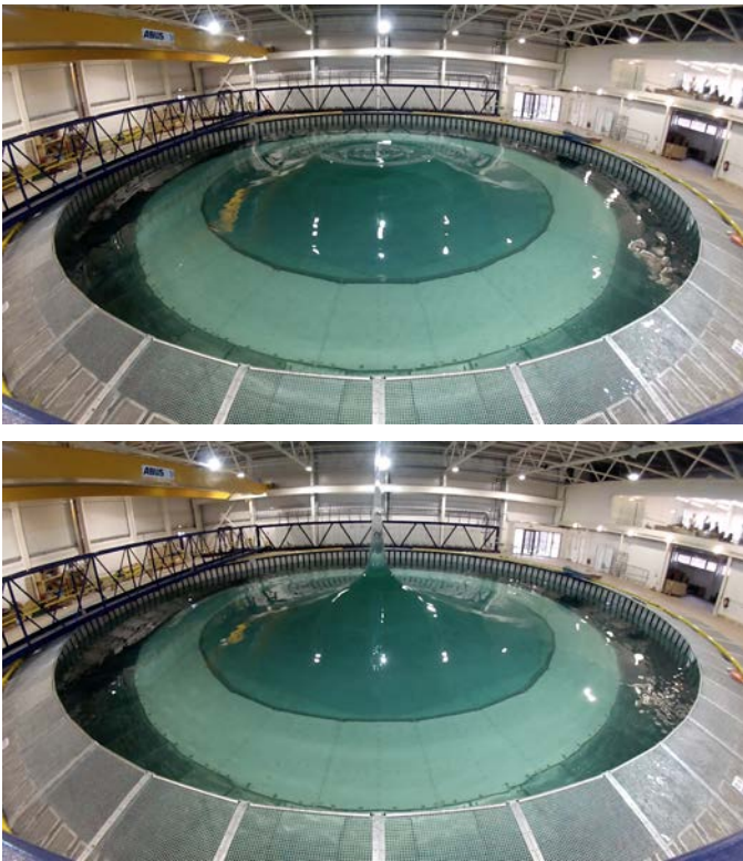
Fig. 16. Focussed breaking wave in the centre of the basin. The top photograph shows phase-locking of the principal wave components approximately 2s before impact, while the lower photograph shows the rapidly up rushing column of water, shortly after impact.
