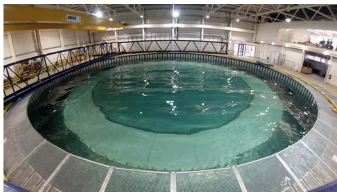
Fig. 15. Pseudo-random waves generated using a JONSWAP spectrum ( T_p = 2\text{s} , H_{m0} \approx 300\text{mm} , \gamma = 3.3 ) with a uniform propagation direction of 270^\circ and a 30^\circ cosine spreading function.
