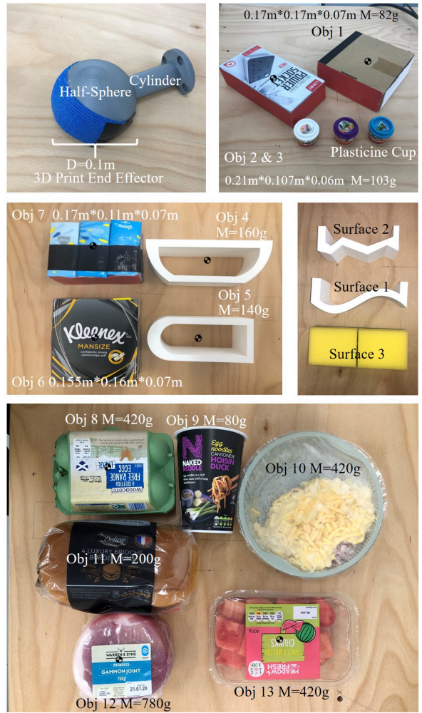
Fig. 6: End-effector, target objects, and support surfaces. Top left: 3D Printed end-effector with blue bandage to increase friction. Top right: object 1, 2, 3 with varying size and mass; plasticine cups for changing the objects’ mass and as disturbances. Middle left: object 4, 5, 6, 7 as target object. Middle right: support surfaces 1 & 2 with curve shape and zigzag shape respectively; sponges as deformable support Surface 3. Bottom: a box of eggs (Obj 8), a cup (Obj 9), a filled bowl (Obj 10), a bag of bread (Obj 11), a cylindrical-shaped ham (Obj 12), a full plastic container (Obj 13).
