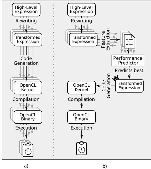
**Figure 1.** LIFT compilation and exploration. a) The current approach compiles and executes all transformed expressions. b) The new strategy ranks the transformed expressions with a model and only compile and execute the best ones.
