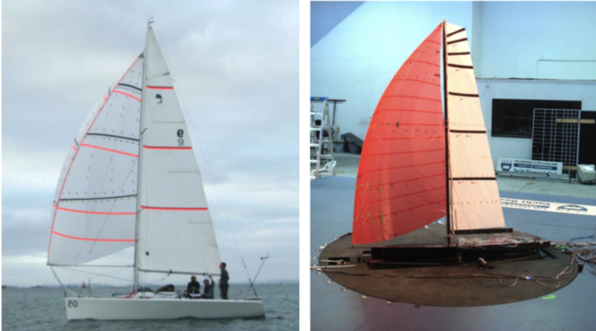
Figure 2: Downwind sailing configurations for the pressure measurements: on-water (Platu-25 left) and wind tunnel (right). In the full-scale tests, the mainsail was reefed slightly in order to align the top of the spinnaker and mainsail to the same height
