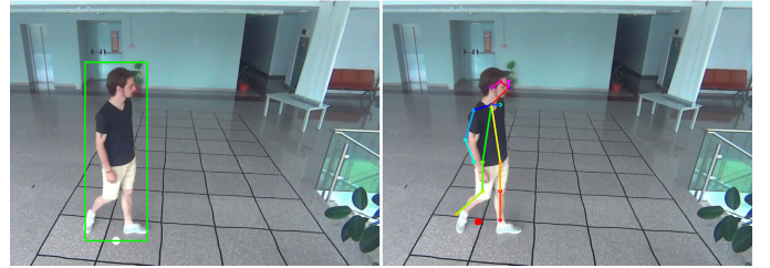
Fig. 1: Position estimation in the 2D-space in front of a camera indicated by the lower white dot using bi-box [3] (left) and our system, CamLoc, based on pose estimation (right).
