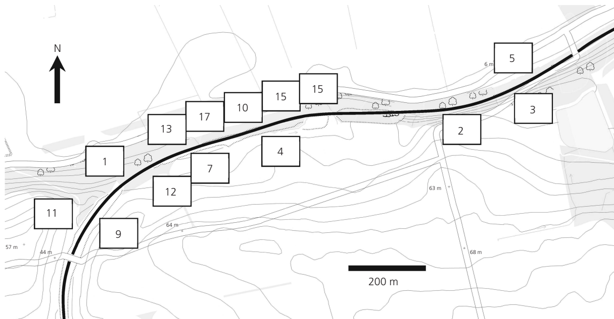
Figure 3. Earthworks prioritisation based on Network Rail weightings. Base map © Crown Copyright/database right 2013. An Ordnance Survey/EDINA supplied service
