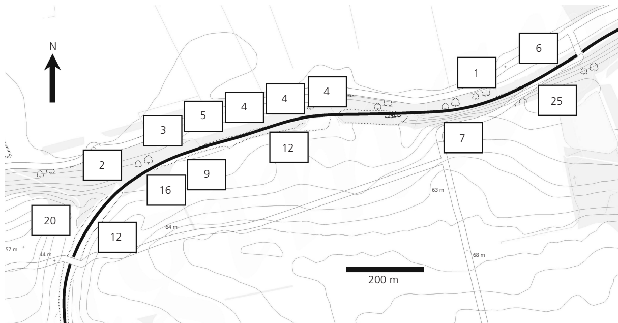
Figure 4. Earthworks prioritisation based on Heritage Railway weightings. Base map © Crown Copyright/database right 2013. An Ordnance Survey/EDINA supplied service
