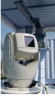
Fig. 3. Sensor setup for collecting real data with the IRST system in the foreground and radar in the background. © Crown copyright, 2019.
